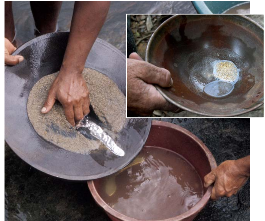
A miner pours the mercury and gold mixture into a tub to be processed. Handling mercury is extremely dangerous. (Inset) After processing tons of soil, a miner shows how much gold he has found in one day.
